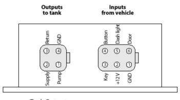
Tank Outputs: 1,2,&3 will provide +12 V when active Vehicle Inputs: 1 must be grounded; do not rely on box mounting screws. 2 +12V batt (always on) through a 15 A fuse 3 looks for +12V when engine is running 4 ground to activate manual purging 5 +12 V output to indicator lamp 6 GM boxes: ground to start purge cycle Ford boxes: +12 V to start purge cycle
