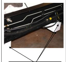
Heat shield mounted to lower tank supports using 6 1%" bolts on the primary tanks or 4 on the secondary tanks. Use pre-existing holes in the lower part of the tank supports.
