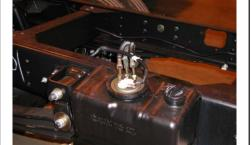
Disconnect electrical connector, hoses and remove temporary gasoline tank from frame rail
